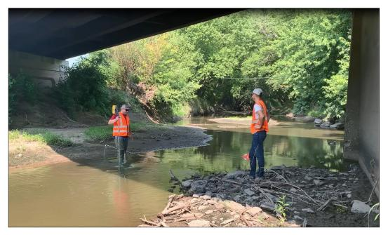
Water Administration team members collect and review stream flow data from more than 200 stations located on streams, rivers, canals, and reservoirs. This data is used both internally and by state and federal agencies for water administration, integrated water management, dam safety, floodplain analyses, and flood warning and emergency response.
