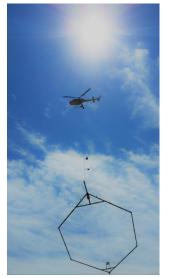
In order to develop a 3D hydrogeologic framework of eastern Nebraska, Eastern Nebraska Water Resources Assessment (ENWRA), through funding obtained through the Water Sustainability Fund, used Airborne Electromagnetics (AEM) to collect subsurface information of the aquifers in the region.
